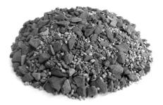
Mineral Substrate for extensive green roofs in single- or multilayered construction
