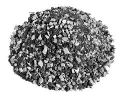
System Substrate for extensive green roofs in single- or multilayered construction.
