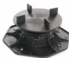
Elefeet® H 30 adjustable from 30–65 mm
