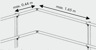
The distance from the joint to the post is max. 0.44 m on the one side and max 1.65 m on the second side.
