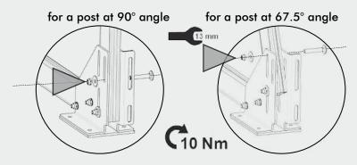
Fit washer and nut and tighten.
