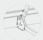
Insert four hammer head bolts into the T-groove of the toe board and insert into the drill holes of the metal brackets on the post. Then, fit the nuts and tighten.
