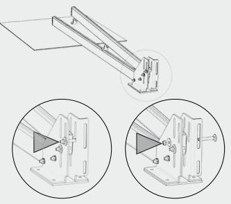
Loosen the marked nuts and remove the bolt.
