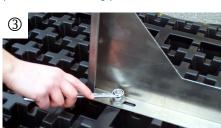
Tighten the screws, tightening torque > 20 Nm.
