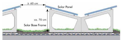
distributed from there in both directions. In this case, a rather lush vegetation can be expected under the solar panels. The plants are relatively easy to access from the walkways between the panels because the panels have their maximum distance of approx. 70 cm to the substrate surface there.
