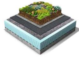
With inverted roofs, layers that prevent the diffusion of damp must not be installed above the XPS thermal insulation boards. Therefore, the water retaining protection mat must be replaced by the diffusion permitting Separation Membrane TGV 21. In the case, that root barriers are necessary they have to be placed below the insulation boards directly onto the waterproofing. A deeper substrate layer compensates for the water retention capacity of the protection mat.
