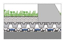
Plug Plants "Sedum Carpet" or Sedum Cuttings System Substrate, depth depends on the superimposed load required ZinCo Solar Base® SB 200 Fixodrain® XD 20 Root Barrier WSF 40, if waterproofing is not root-resistant
