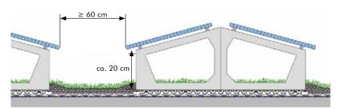
The front edge of the solar panels has a sufficient distance to the substrate surface so that plants can still grow under the panels.
