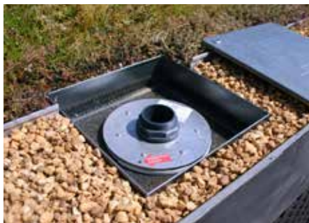
The flow controller is protected beneath the inspection chamber and regulates the slow discharge of water. At the same time, it acts as an overflow.
