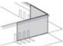
Creation of an internal corner with corner connector
