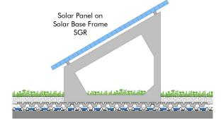
Plant layer "Sedum Carpet" System Substrate "Sedum Carpet" ZinCo Solar Base SB 200 Fixodrain® XD 20
